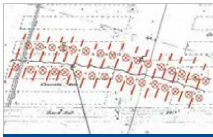
Historic bridge, Christchurch, NZ Longitudinal crack repair schedule
