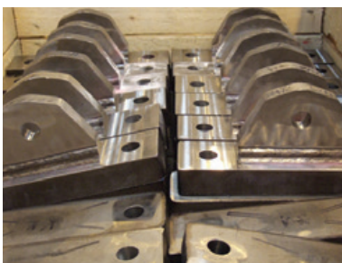
Tunnel Ceiling Suspension Systems
