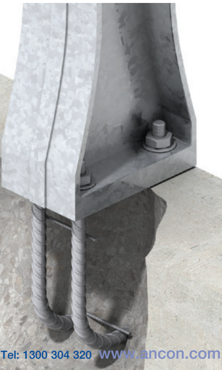
Engineered Reinforcing Bar. Project: Cradlewell Bypass, UK (Contractor: Alfred McAlpine/Carillion)
