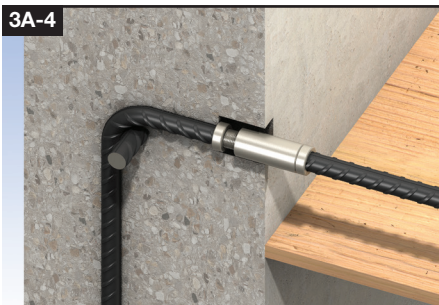
Position the continuation bar with the coupler against the end of the fixed bar.
