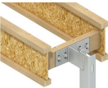
Top Connection of a WP3 Windpost to a Side-Fixed Timber Noggin
