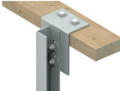
Top Connection of a WP3 Windpost to the Top of a Timber Wall Plate
