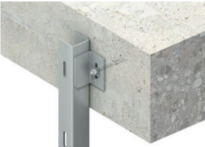
Top Connection of a WP3 Windpost to the Face of the Concrete
