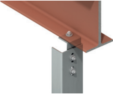
Top Connection of a WP2 Windpost to the Underside of a Steel Beam
