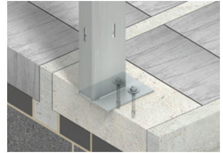
Base Connection of a WP2 Windpost to a Concrete Infill in the Top of a Beam and Block Floor
