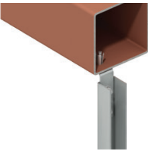
Top Connection of a WP3 Windpost to the Underside of a Steel Box Beam
