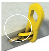
Anchor bearing crack
