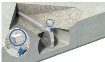
Anchor sheared by the clutch
