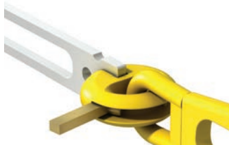
Conventional clutch has a round locking ring so the clutch is free to rotate around the anchor under shear load.
